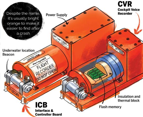
**! Built to survive extreme conditions,** black boxes can endure forces up to 3,400 Gs, temperatures reaching 1,100°C, and transmit signals every second from depths of up to 19,000 feet for as long as 30 days.
