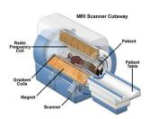
The MRI scan works on the principle of Nuclear Magnetic Resonance or NMR. It uses the fact that the nucleus of atoms spin and have an electric charge produces a magnetic field (just like current in a magnet).
