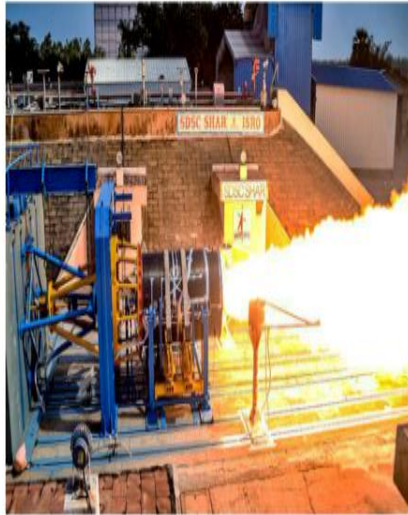
Kalam-250, the second stage of Vikram-1 launch vehicle, being test
